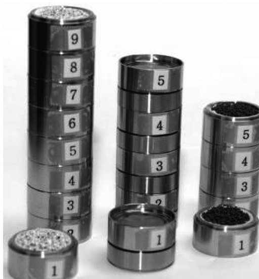
Figure 2. Filter media includes zeolite (center) and aluminosilicate (left, right) based materials.
